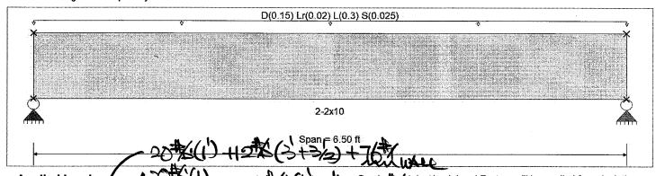
**Applied Loads** Beam self weight calculated and added to loads d. Load Factors will be applied for calculations.
