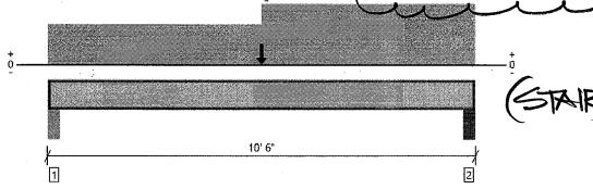
All locations are measured from the outside face of left support (or left cantilever end). All dimensions are horizontal.
