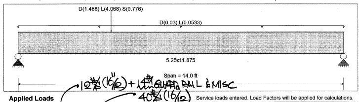
Beam self weight calculated and added to loads
