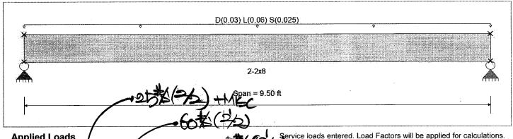
**Applied Loads** Beam self weight calculated and added to loads
